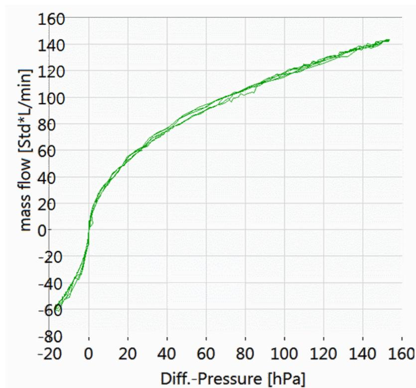
**Figure 1:** Data of several inhalations for correlation curve before building process
