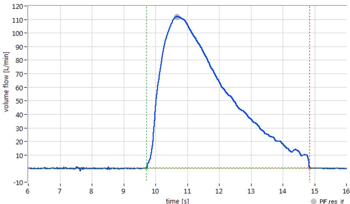
**Figure 2:** Inhalation curve of a tested DPI with volume flow versus time
